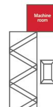
Machine room in ordinary machine room elevator
